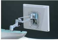
21 LCD monitor arm (Three-point vertical control) JJA-LA21 This arm holds a LCD monitor, size up to 15-inch (approximately 5kg or less, 65mm or less in thickness). Mount specification: 75 x 75 VESA
